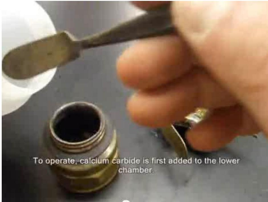
To operate, calcium carbide is first added to the lower chamber.
